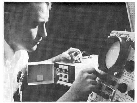
A PORTABLE CHARGE SOURCE is held by Eugene R. Fisher of Environmental Test Area I, 8111. Mr. Fisher developed the battery-powered instrument to check out the operation of charge amplifiers which are used in data collection for various types of environmental tests. Previously such check-outs required more unwieldy and cumbersome equipment which created problems during tests outside of a laboratory.
